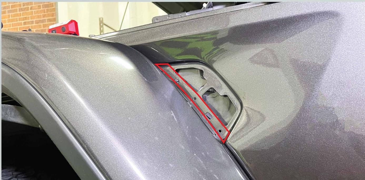
9. Pull back the backing off of the double sided tape. and install the side marker onto the fender.
