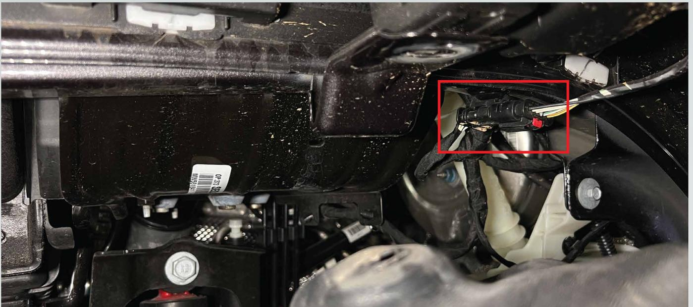
4. With a plastic pry tool, pry out the fender vent in the order shown below.
