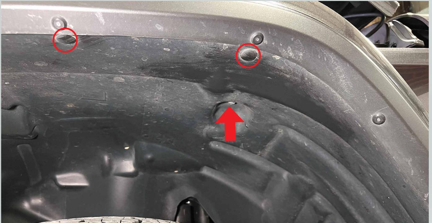
3. Pull the fender liner down and locate this connector toward the middle of the fender. Unplug it by sliding the red tab back, then press the release tab down, and slide the connector apart.
