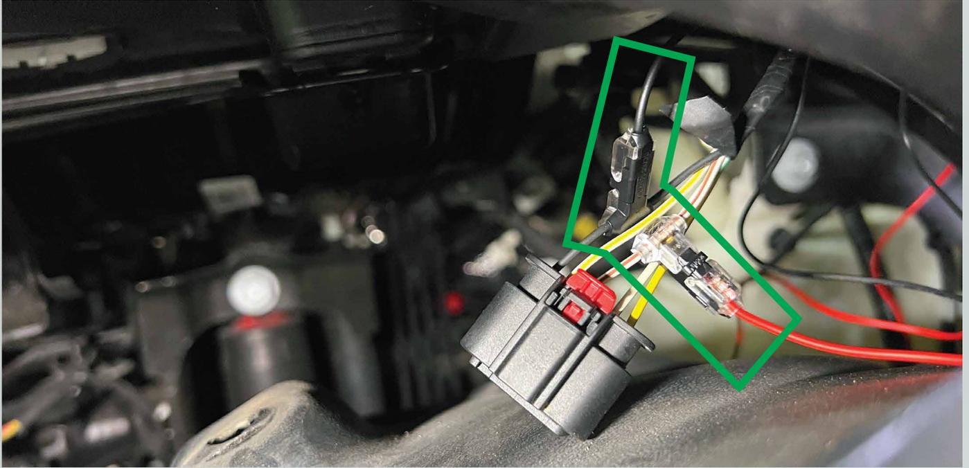
11. Plug the fender wiring back into the vehicle wiring and reassemble the fender liner in the reverse order that you took it apart.
