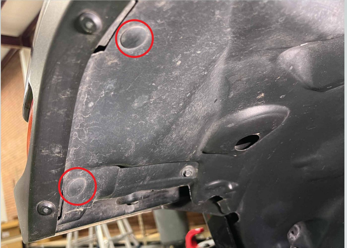
2. Towards the back of the fender, remove this (1) one 10mm bolt, and (2) two push clips.
