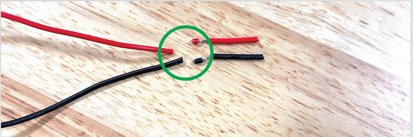
6. Get one of the included wire taps , insert the wire into the tap, and crimp down the cover with pliers until the cover locks into place. Repeat on the other wire.
