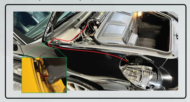
9. With the headlight removal tool still inserted on the driver side, grab your driver side Morimoto headlight, bring it to the car and plug in the DRL harness. Next line up the guide pins on the sides of the headlight with the channels on the vehicle and slide the headlight into it's place. With one hand turn the tool clockwise while pressing the headlight into the fender with the other hand. Carefully turn the tool til you hear a pop sound.
