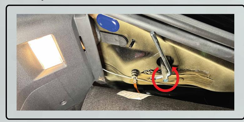
6. Remove the battery cover by rotating the two (2) plastic screw 90 degrees counter clockwise. Then simply pivot the front edge of the battery cover up and take the battery cover out of the car. Then remove the panels labeled #1, #2 in the picture. To remove them simply lift them up and out of the car.
