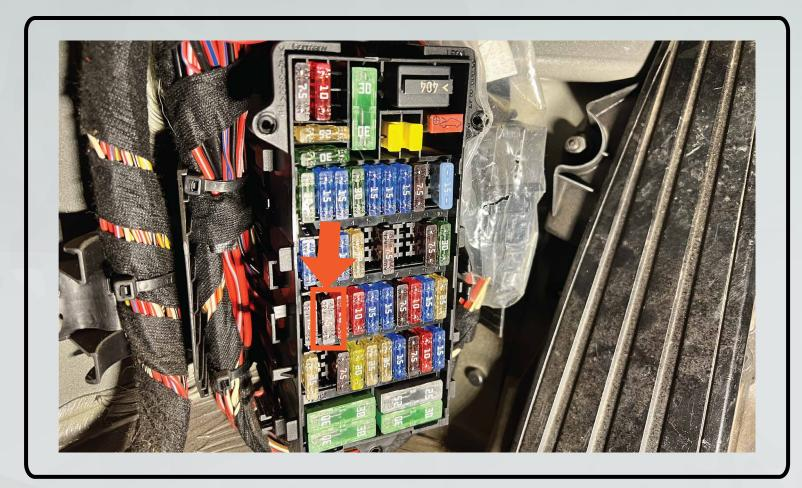
16. Back under the hood, connect the other end of the Fuse Tap Harness to the DRL Harness.
