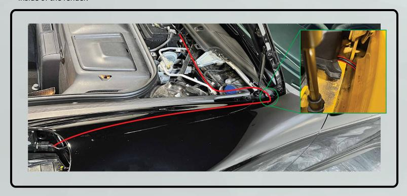
8. Route the passenger side DRL Harness as pictured below. Run it under the windshield cowl and into the inside of the fender. using a wire snake run it along the top channel on the inside of the fender.
