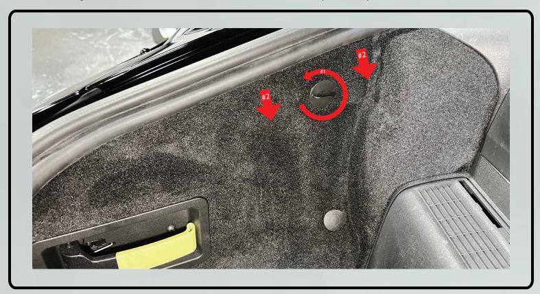
2. With the liner pulled back, remove this rubber plug. Do this by simply pulling it away from the sheet metal. Repeat steps #1, 2 on the other side of the car.
