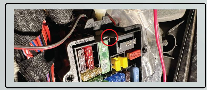
15. Remove fuse C2 7.5 A fuse and plug in the Fuse Tap Harness in place of that fuse. Reassemble the kick panel.
