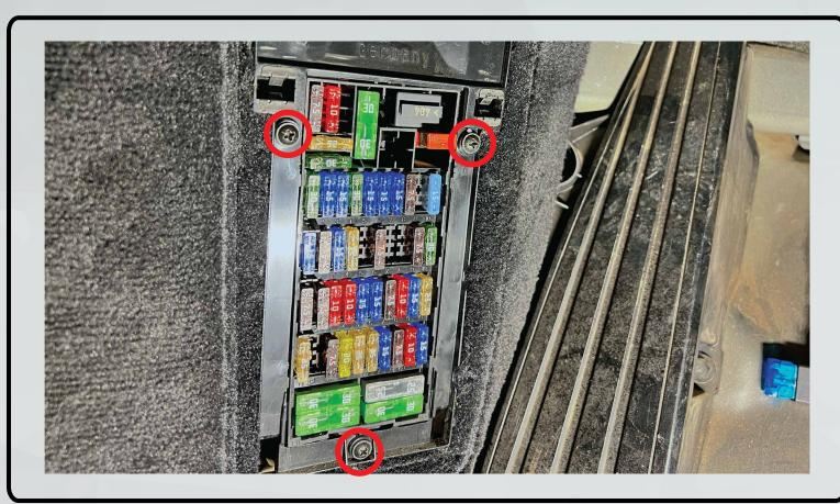
14. At the top of the fuse box cut out a small slot for the Fuse Tap Harness to pass through. We used a pair of diagonal wire cutters to make the slot.
