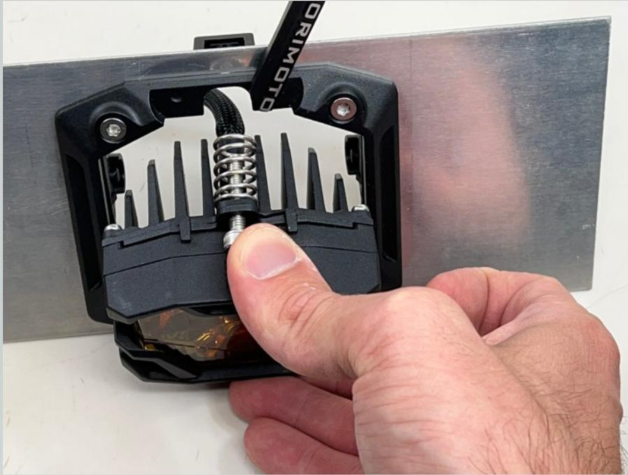
10. Open the adjuster door on the front bezel. Making sure that the spring does not fall off the back of the screw, insert the pod through the bezel and onto the mounting bracket. Get the adjuster screw started into the adjuster threading clip. Turn the adjuster screw 5-6 turns but do not tighten down.
