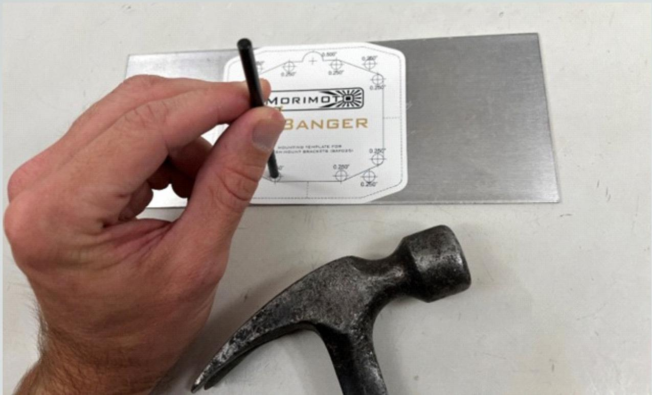
2. Remove the template and drill holes at each location indicated by your punches. As indicated on the template, 12 holes are 0.25" / 6mm diameter and the top center hole is 0.50" / 13mm.
