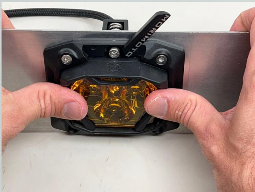
12. Finally, insert the bottom two front bezel to mounting bracket screws and tighten all four screws. Use the adjuster screw to aim the pod to your desired vertical angle. Tightening this screw will adjust the pod to aim higher, loosening will aim down.
