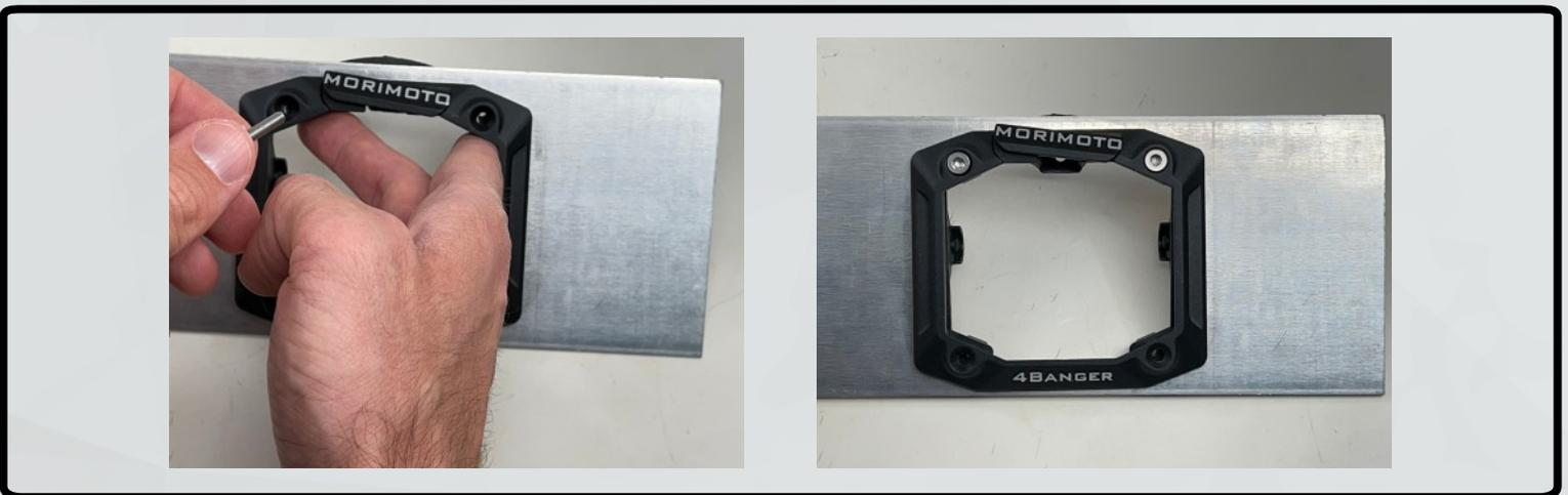
7. Prepare your 4Banger pod for installation by attaching the adjuster bracket. First, remove the top two screws from the back of your pod using a Torx T10 bit (note the top of the pod is indicated by the "M" logo.)
